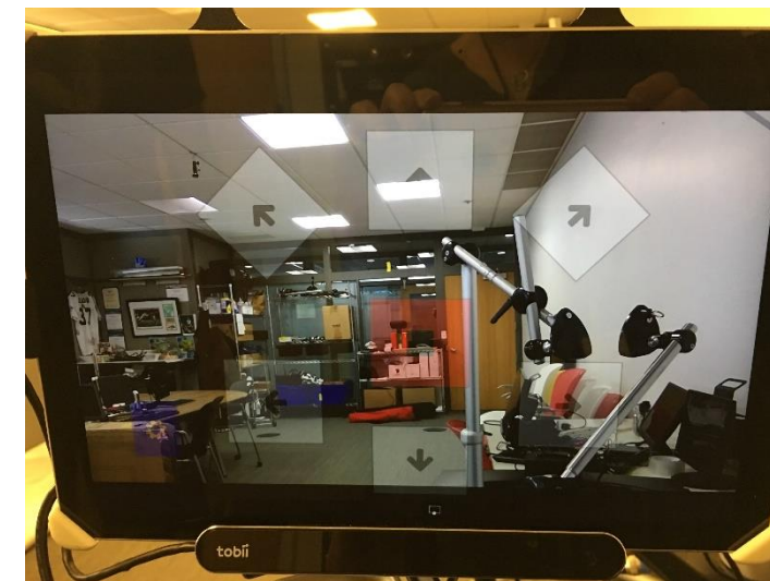
Figure 2: Eye-gaze system user interface. Gazing at the arrows allows user to direct the PWC while seeing their environment.
