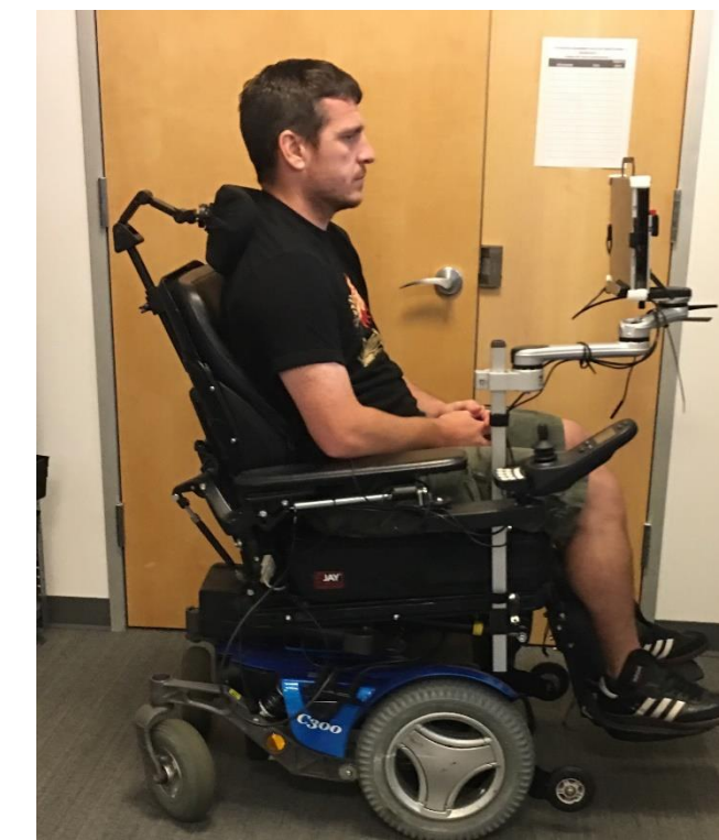
Figure 1: Eye-gaze system on power wheelchair
