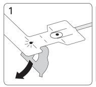
1. Remove the backing from the sensor.
