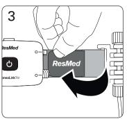
**3.** Fasten the tab to the belt. Slide the device into a position that is close to the effort sensor.
