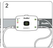
2. Check that lights next to the accessories you are using are green. If any of these lights are red and blinking, the accessories are not attached correctly.
