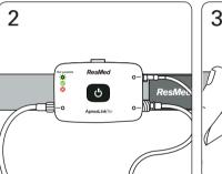
2. Check that the test complete indicator light is lit and green. This means the test is complete. If the test indicator light is red, replace the batteries and repeat the test tomorrow night.
