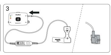
3. Attach the oximeter to the oximeter connector on the device by pushing it on.
