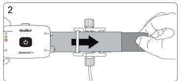
2. Flip the device over. Thread the end of the belt closest to the device through one of the slots on the effort sensor (if used).
